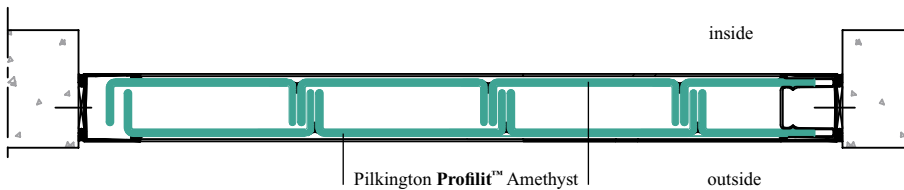
Vertical double-glazed installation Horizontal section
